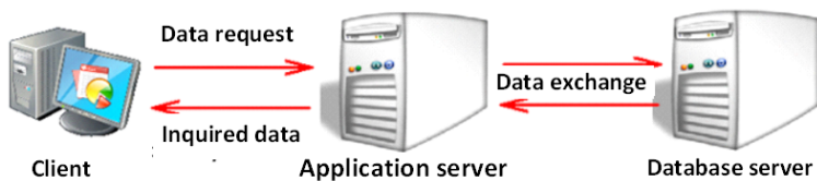
Fig. 1.8. Client-server three-tier architectures
