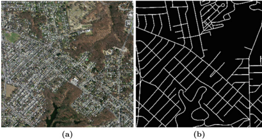
Fig. 4 a Input raw image of road map, b Corresponding ground truth image
