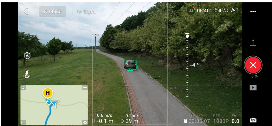
**Fig. 3. DJI Fly graphical interface that allows you to mark an object for tracking.**
